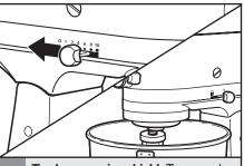
To place pouring shield: Turn speed control to "O". Unplug Stand Mixer. Attach your chosen accessory, see "Attaching/removing the flat beater, wire whip, or dough hook" section.
