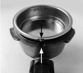
To add or remove the filter from the portafilter, line up the raise dot on the side of the filter with the gap on the side of the portafilter.
