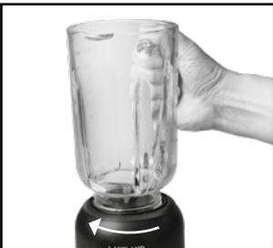
4. Sit the glass blending jug onto the main unit. Turn it to the left so it locks onto the main unit.
