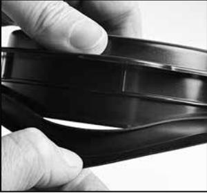
1. To reapply the seal, make sure the seal has the two sealing strips on the outside.
