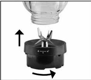
3. This then screws anticlockwise into the base of the glass blending jug.
