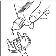
The bamix will stay longer "fit" if you oil it every few months. For this use an acid-free oil (e.g. vaseline oil, obtainable at a chemist's). Hold the bamix upside down with the cutter guard facing you, put 2 or 3 drops of oil on the drive shaft, and switch on the appliance for 2 to 3 minutes. Afterwards rinse the appliance in hot water.
