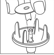
Push the attachment as straight as possible on to the stub in such a way that the drive pin on the stub fits exactly into the small recess in the socket of the attachment. The attachment is designed to make this process easy. The attachment is removed by simply pulling it off from the stub. For protection please use a cloth.
