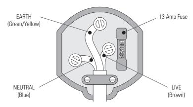
Ensure that the outer sheath of the cable is firmly held by the clamp.
