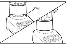
**NOTE:** If there is a gap between the locking collar and the base, the pitcher (or culinary jar) might not be locked into the locking collar or the assembly may not be positioned properly on the Blender base. If necessary, repeat steps 1 through 4.
